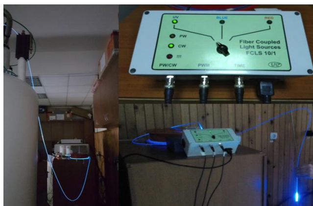
Figure 1. The setup for in situ irradiation NMR spectroscopy.
